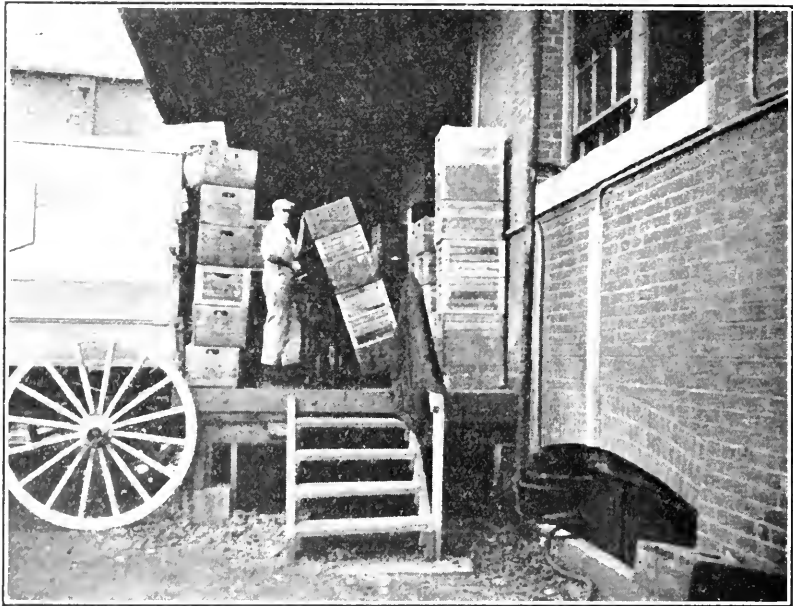
FIGURE 11. Checking in routes at a plant using system 10. An average of only 9.7 routes per hour and 3.2 routes per man-hour was checked in at four plants using this system.
